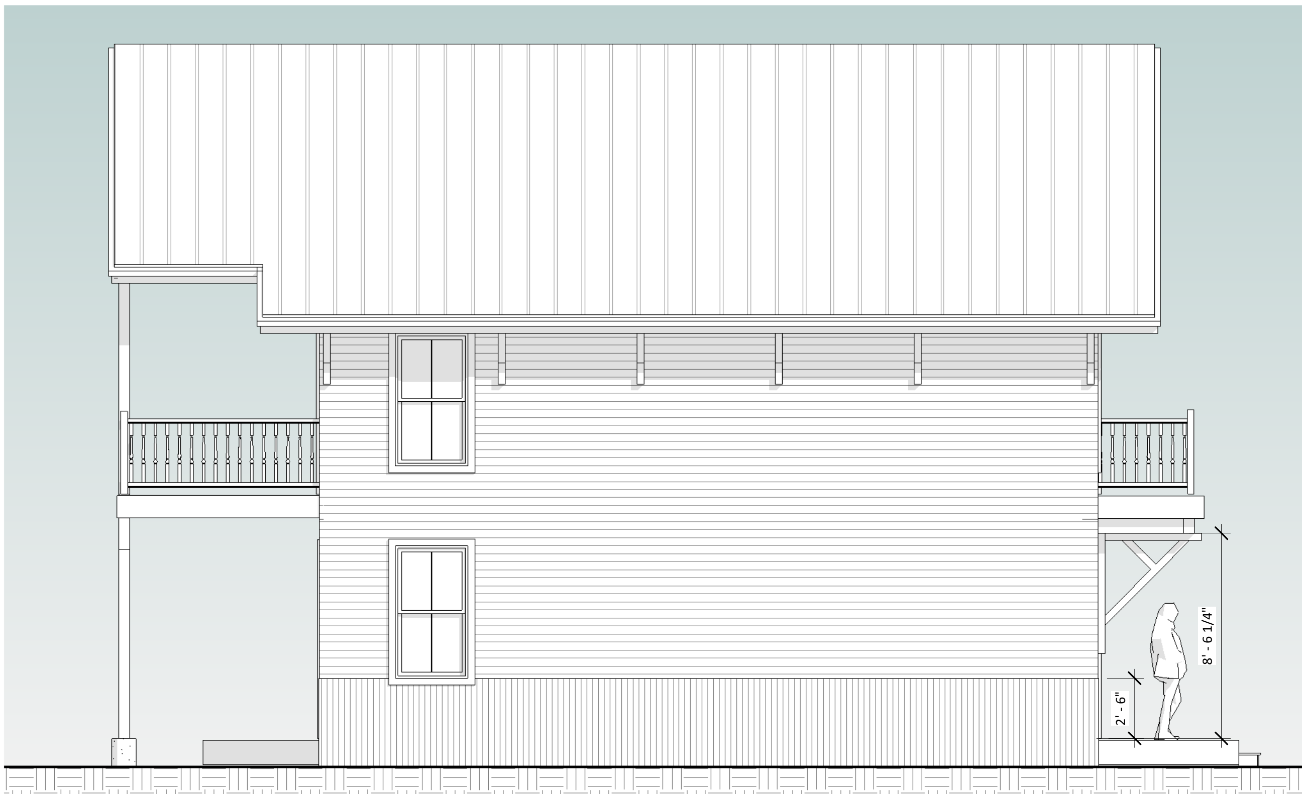
2 NORTH EAST ELEVATION 1/4" = 1'-0"
