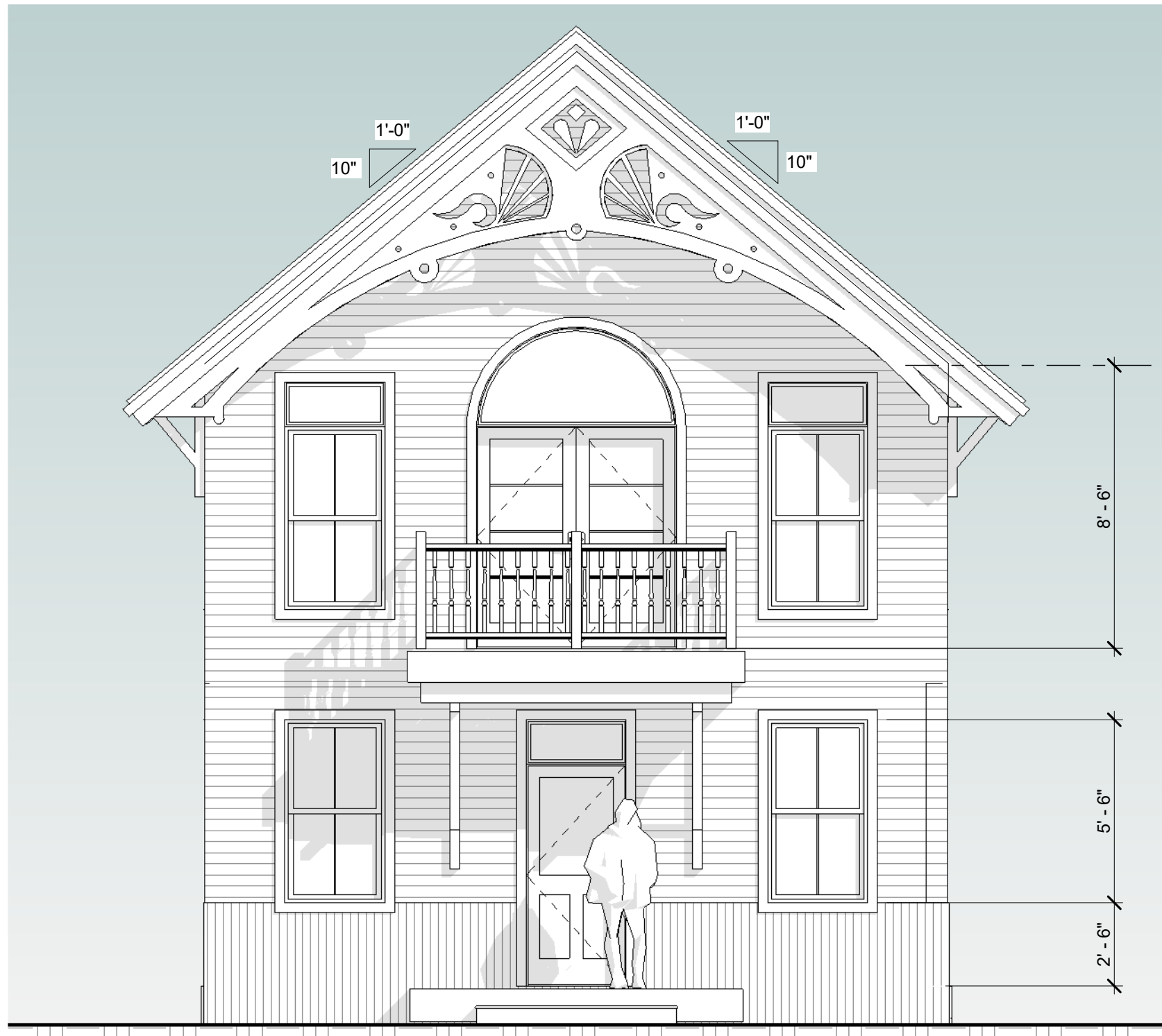
4 NORTH WEST ELEVATION 1/4" = 1'-0"
